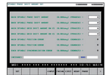
Shift amount setting for spindle phase synchronization control
