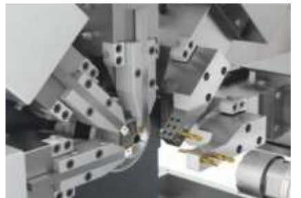
Back spindle The back side is a type 12 spindle, using the spindle end drill process
