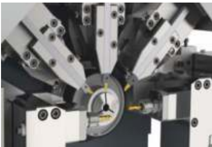
Bilateral milling mode Both 1 and 5 knife racks can be installed with one side power
