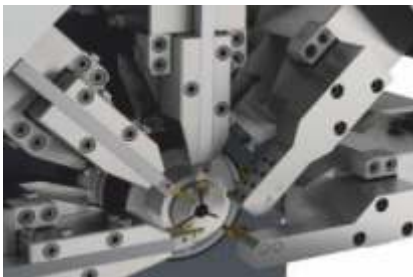
Multi-knife mode The double knife holder and porous drilling arm combination can be installed with up to 13 cutting tools.
